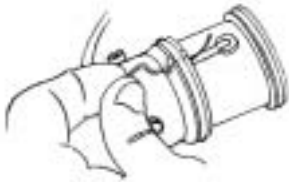
3.5 Untie and remove the ground strap (12)
