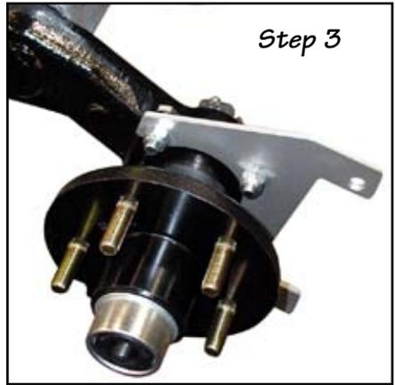
4. Place cap style rotor over hub. Make sure the hub face is clean with a smooth surface or:
