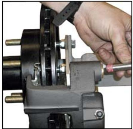
5. Place caliper over rotor and mounting plate. A bleeder valve must be in the up position (see below). Check both calipers for this position. Some calipers have two valves others have only one.
