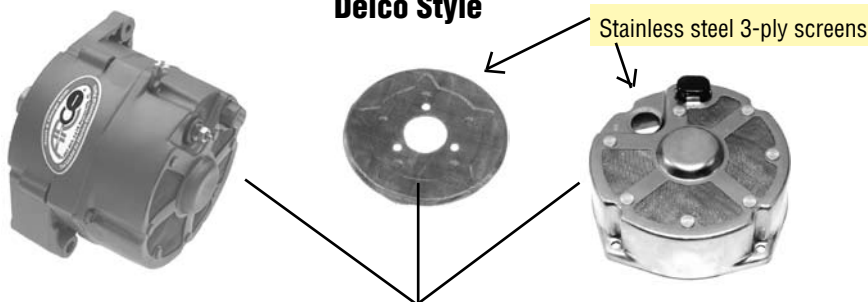
Delco style alternators use flame arrestors instead of sealed brush compartments.
